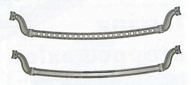
The overall strength of the Hoffman axles is considerable higher than all others that were tested. Of the axles tested by Hoffmans (the good ones) were around the 400Mpa point, while theirs is 568Mpa.
