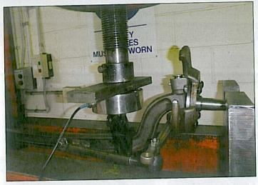
Jigs were made to complete these tests and with the help of a local and very helpful TAFE they were able use their 100T press to undertake these tests.
