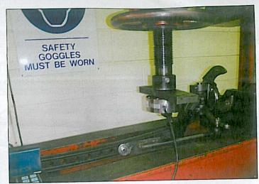
from this test is that Hoffmans deliberately elected to test what was potentially their weakest axle, the longest version with drilled beam. In the case of the axle itself, it actually tested safely to double its certified strength. It would have to be a very big street rod to have a front end load of more than 800 kilograms.
