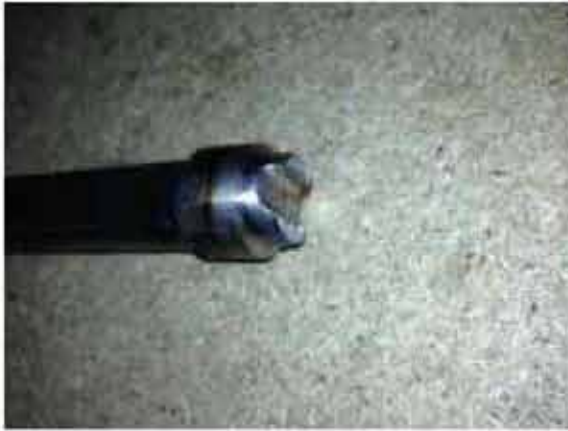
Failed Flaming River Column
