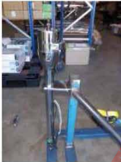
Column installed in test jig
