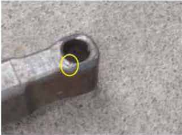
Ford Column post test (crack circled)
