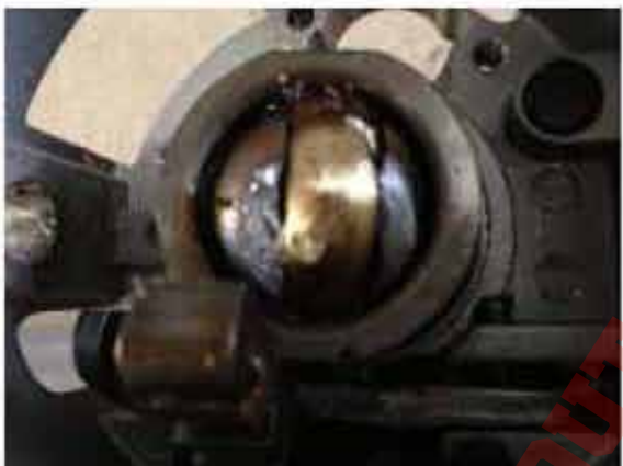
Failed Flaming River Column
